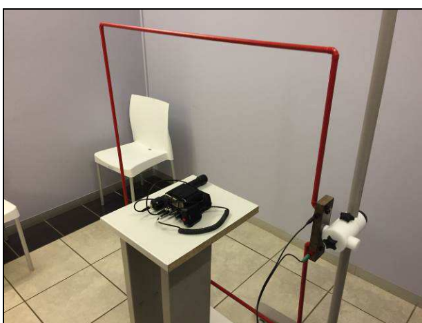
SANS / IEC 61000-4-8: Power frequency magnetic immunity test set-up
